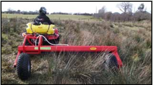
With 60L tank, drawbar shown in offset position
