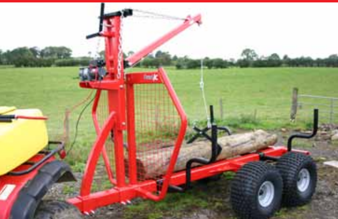
Electric winch and crane shown
