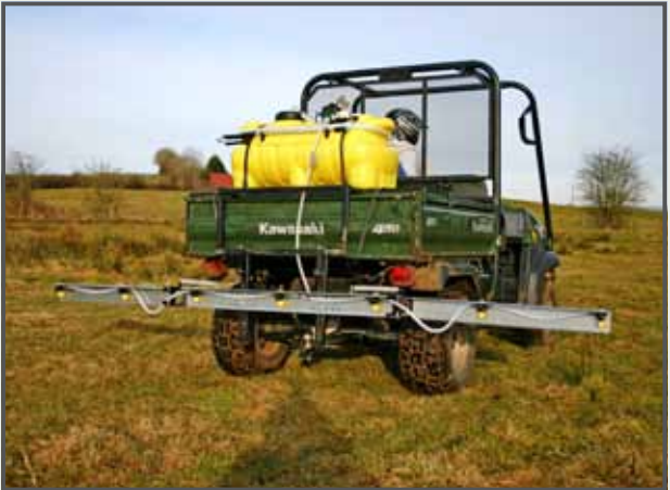
100L pro spray with anti-drift boom shown
