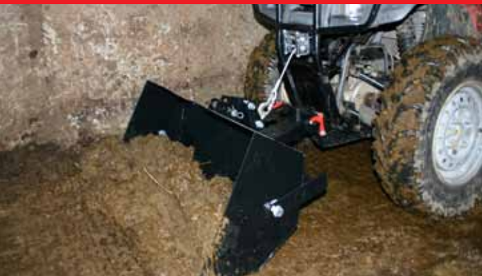
Front Bucket mucking out
