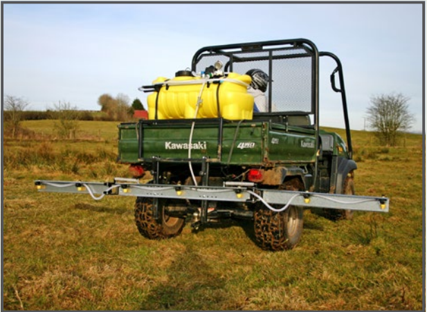
100L pro spray with anti-drift boom shown
