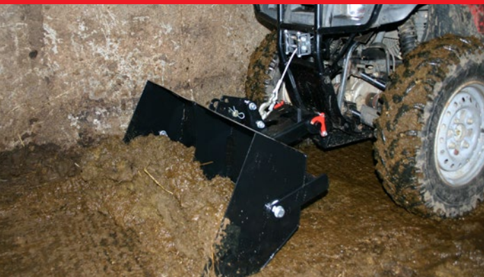
Front Bucket mucking out
