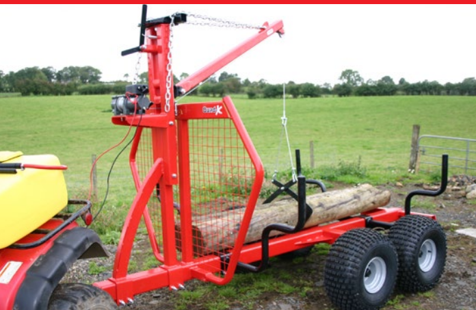
Electric winch and crane shown
